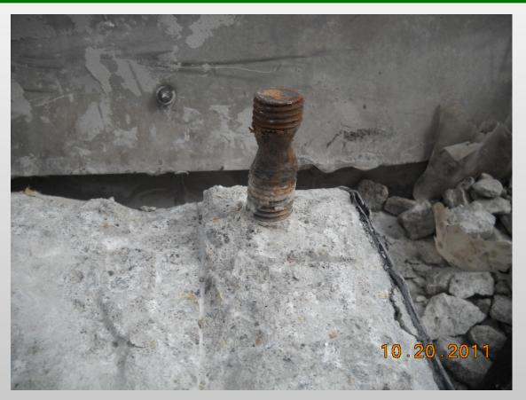
**Dissimilar Materials:** A galvanic reaction occurred due to a lead washer being installed on a carbon steel threaded rod for waterproofing.
