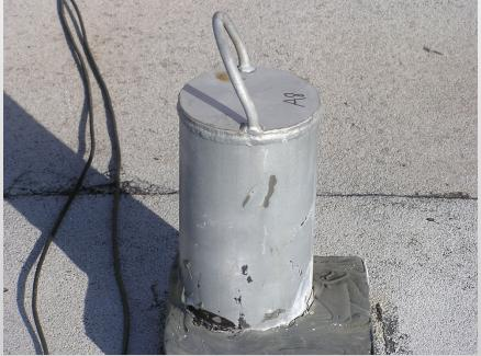
Field Fabricated Anchors: Anchor failed at less than 1,000 lbs. during load testing. OSHA required ultimate load is 5,000 lbs.
