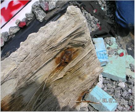
Construction Deficiencies: Plywood anchor rod templates were inadvertently left behind and trapped moisture. This condition accelerated corrosion of anchor rods. The rods failed during load testing.
